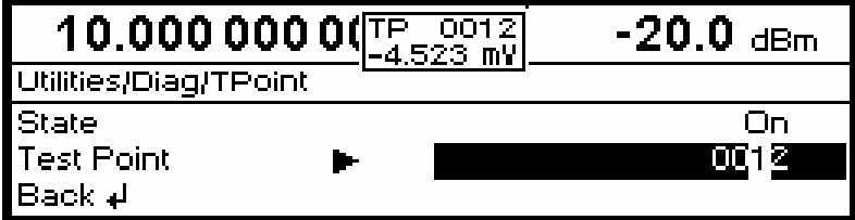
Fig. 4-39 Utilities – Diag – TPoint menu
