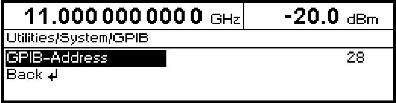
Fig. 4-32 Utilities - System - GPIB - Address menu
